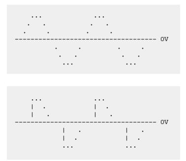
As you can see, by varying the turn-on point, the amount of power getting to the bulb is adjustable, and hence the light output can be controlled.
