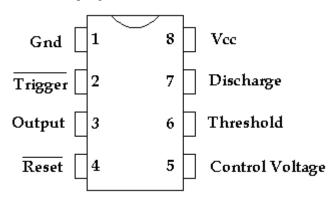
Pin 2 (Trigger) is the 'on' switch for the pulse. The line over the word Trigger tells us that the voltage levels are the opposite of what you would normally expect. To turn the switch on you apply 0 volts to pin 2. The technical term for this opposite behavior is 'Active Low'.
