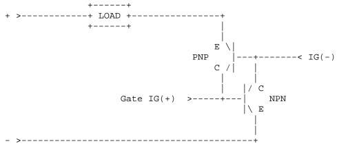
If we connect the positive terminal of a supply to say, a light bulb, and then to the emitter of the PNP transistor and its return to the emitter of the NPN transistor, no current will flow as long as the breakdown voltage ratings of the transistor are not exceeded because there is no base current to either.
